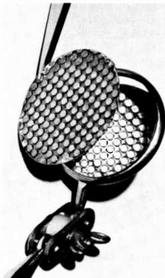
Fig. 12—Back-to-back mesa diodes on wafer (back side of wafer can be seen in mirror).
